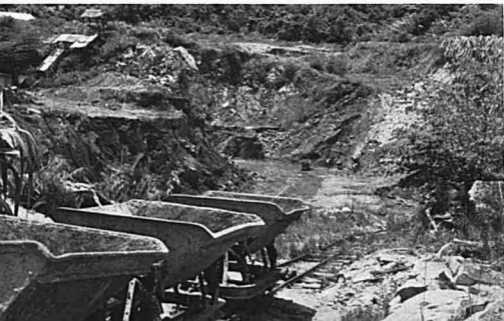
Plate XII Bukit Young Gold Mine, Bau, First Division. The mined ore is shovelled into bucket trucks which are winch-hauled up a light rail track to the plant for treatment by the cyanide process.
